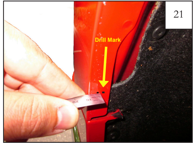
Remove the flare. Using the marks made in step 18 as a guide, measure inward from the outside edge of the fender to verify proper depth of original marked location. Mark must be minimum of 22mm in from outside edge of fender, if short, adjust marks to 22mm.
