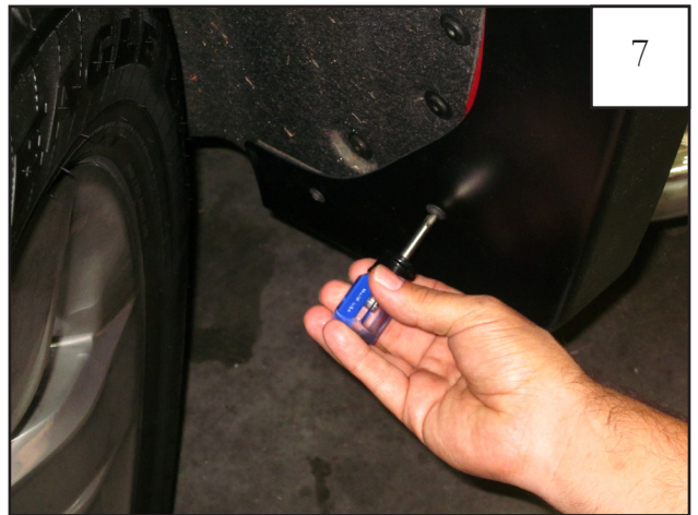
Hold flare in place and start supplied Screws (Item 2) through two bottom rear holes in flare and into factory hole in rear of wheel well. Do not tighten.
