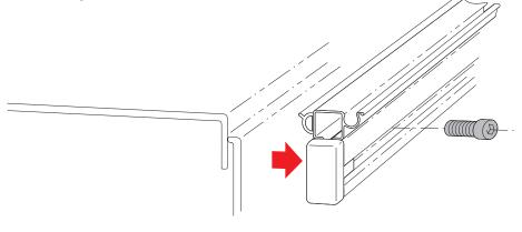
Apply the adhesive foam seal to the inside surface of the factory tie-down rail.
