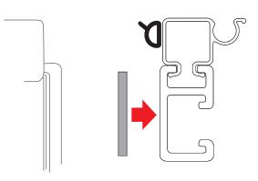
Reinsert the tie-down rail bolt through the foam seal and reconnect the tie-down rail to the truck bed wall.
