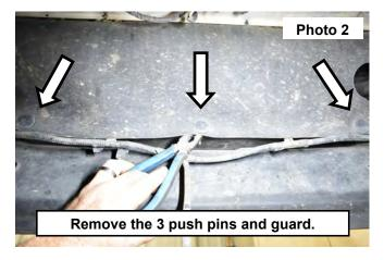
3. Remove the push pins on the inside of the bumper holding the block heater plug to the bumper. See Photo 3 and 4.
